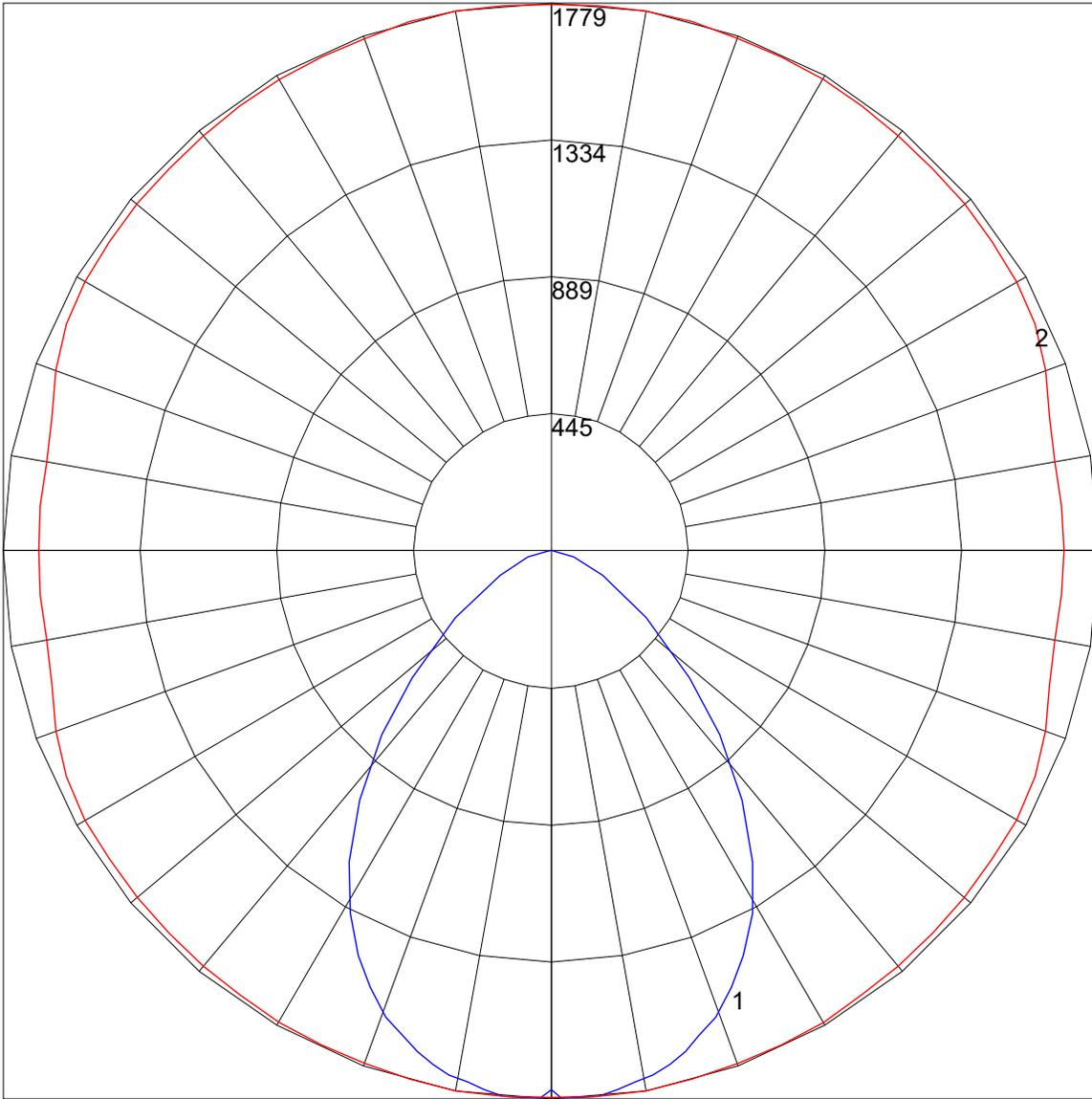
Maximum Candela = 1778.98 Located At Horizontal Angle = 80, Vertical Angle = 3
