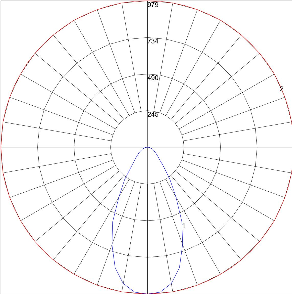
Maximum Candela = 979.2 Located At Horizontal Angle = 0, Vertical Angle = 0
