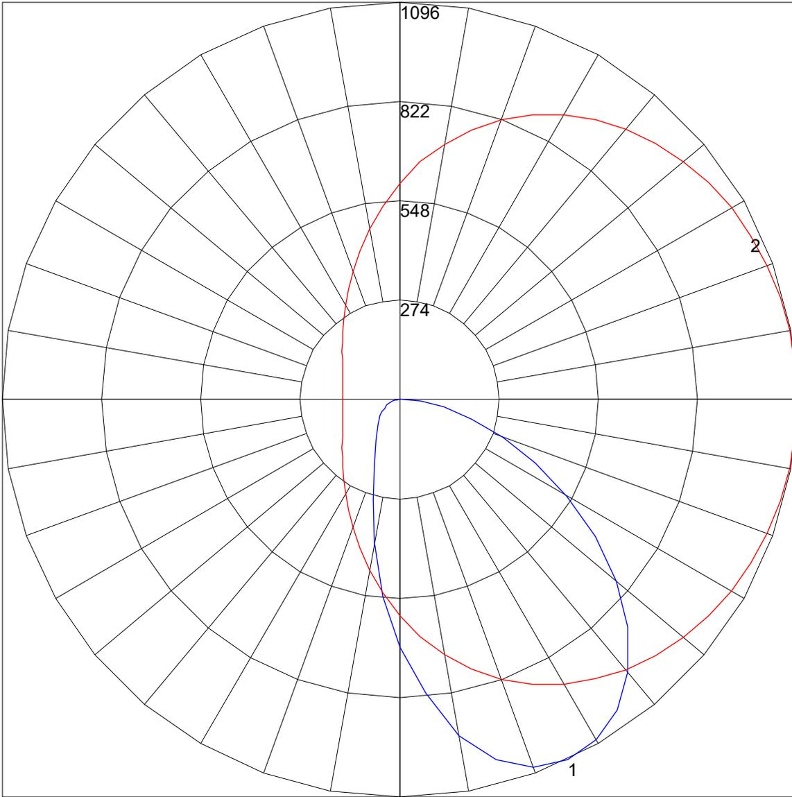
Maximum Candela = 1096.327 Located At Horizontal Angle = 0, Vertical Angle = 25
