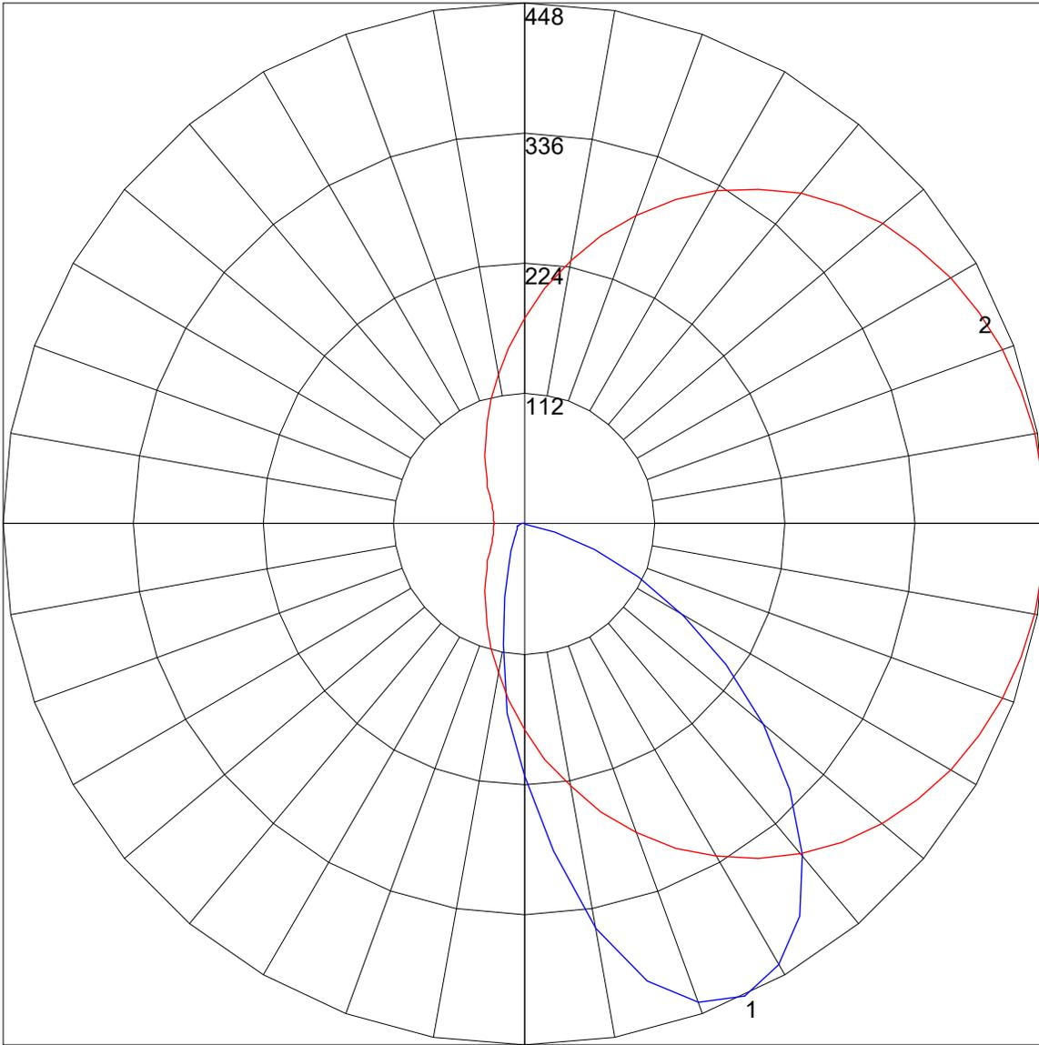
Maximum Candela = 448.37 Located At Horizontal Angle = 0, Vertical Angle = 25
