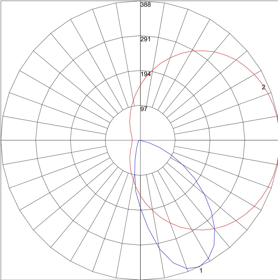
Maximum Candela = 387.574 Located At Horizontal Angle = 0, Vertical Angle = 25
