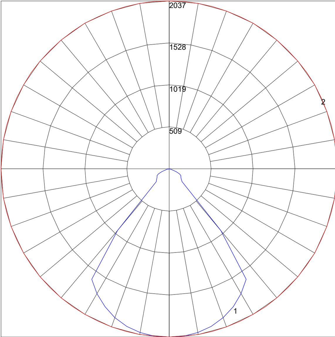
Maximum Candela = 2037 Located At Horizontal Angle = 0, Vertical Angle = 0
