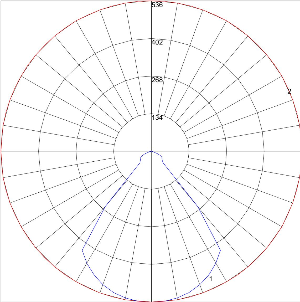
Maximum Candela = 535.5 Located At Horizontal Angle = 0, Vertical Angle = 0
