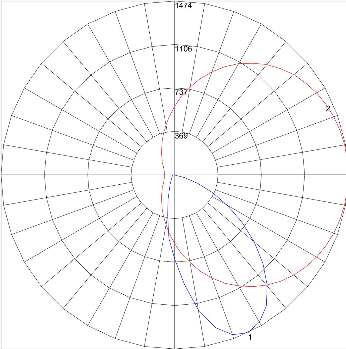
Maximum Candela = 1474.303 Located At Horizontal Angle = 0, Vertical Angle = 25
