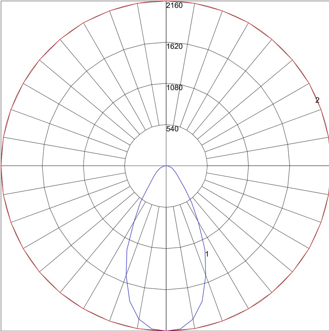
Maximum Candela = 2160 Located At Horizontal Angle = 0, Vertical Angle = 0
