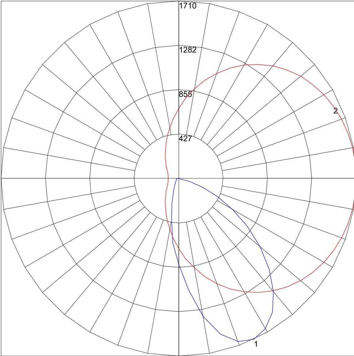
Maximum Candela = 1709.888 Located At Horizontal Angle = 0, Vertical Angle = 25
