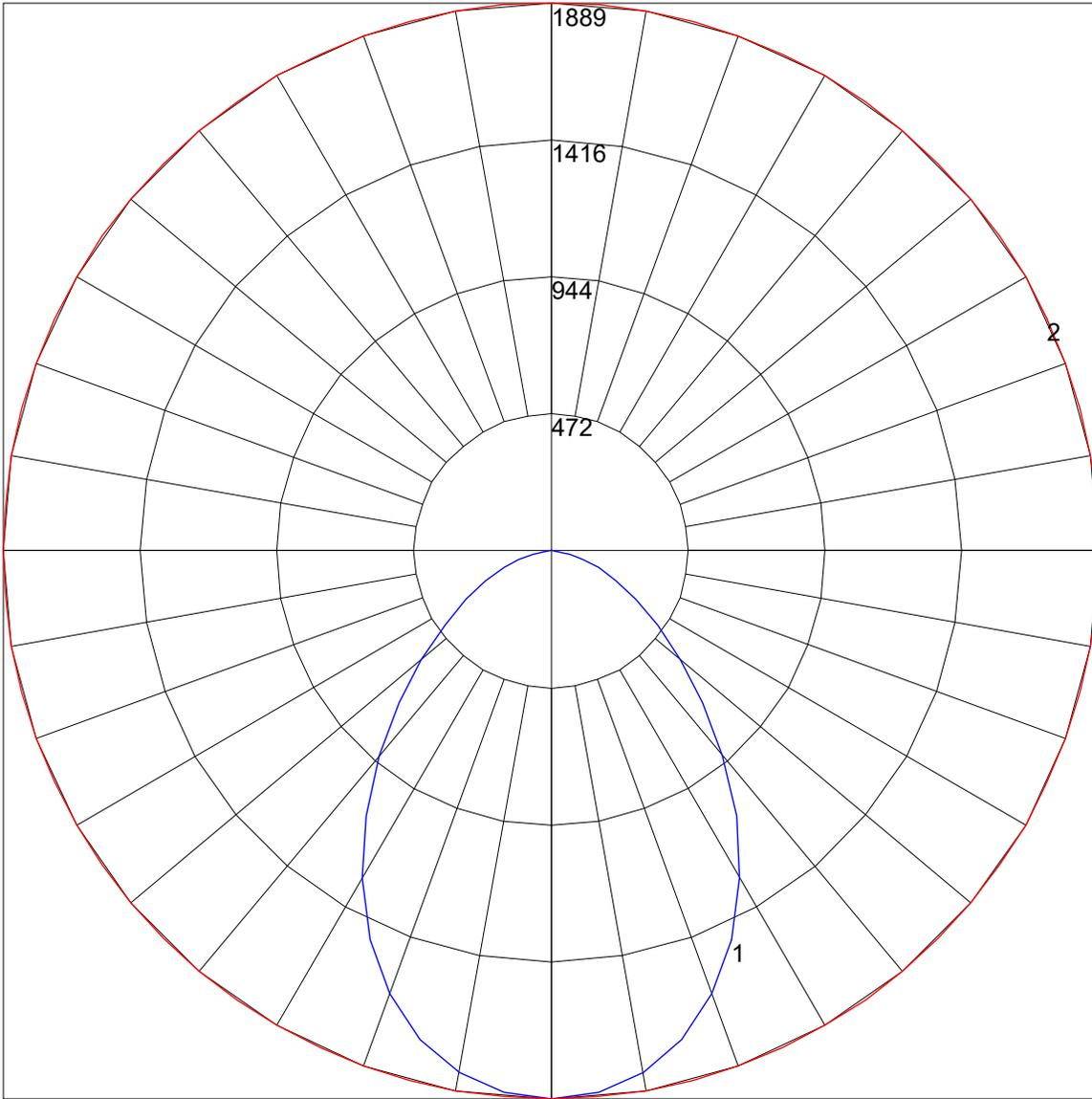
Maximum Candela = 1888.6 Located At Horizontal Angle = 0, Vertical Angle = 0
