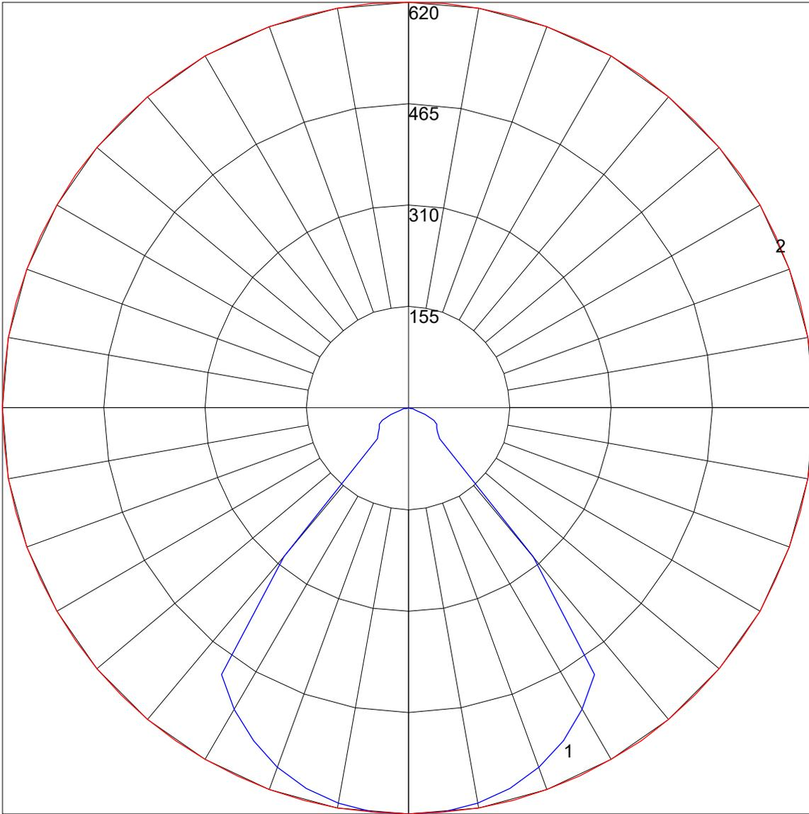
Maximum Candela = 619.5 Located At Horizontal Angle = 0, Vertical Angle = 0
