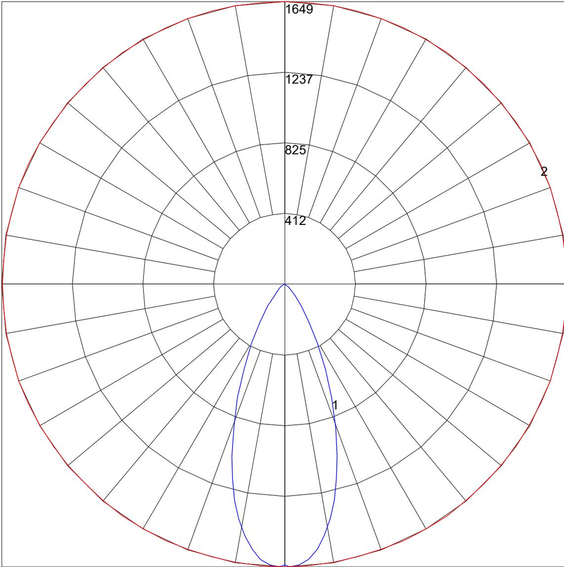
Maximum Candela = 1649 Located At Horizontal Angle = 20, Vertical Angle = 1
