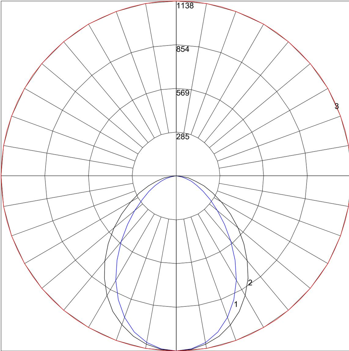
Maximum Candela = 1138 Located At Horizontal Angle = 0, Vertical Angle = 0
