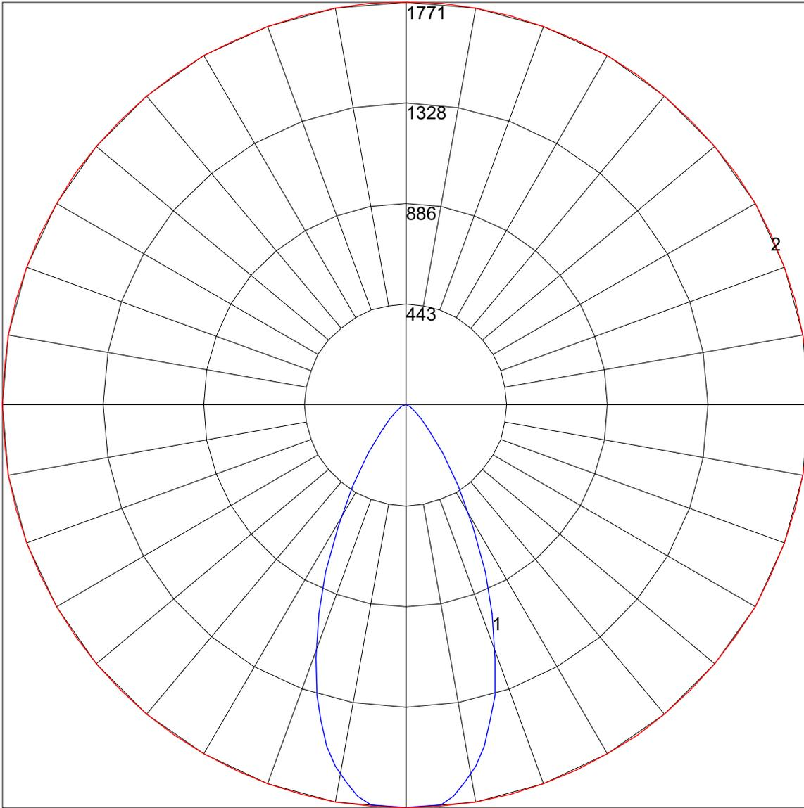
Maximum Candela = 1771.22 Located At Horizontal Angle = 0, Vertical Angle = 0
