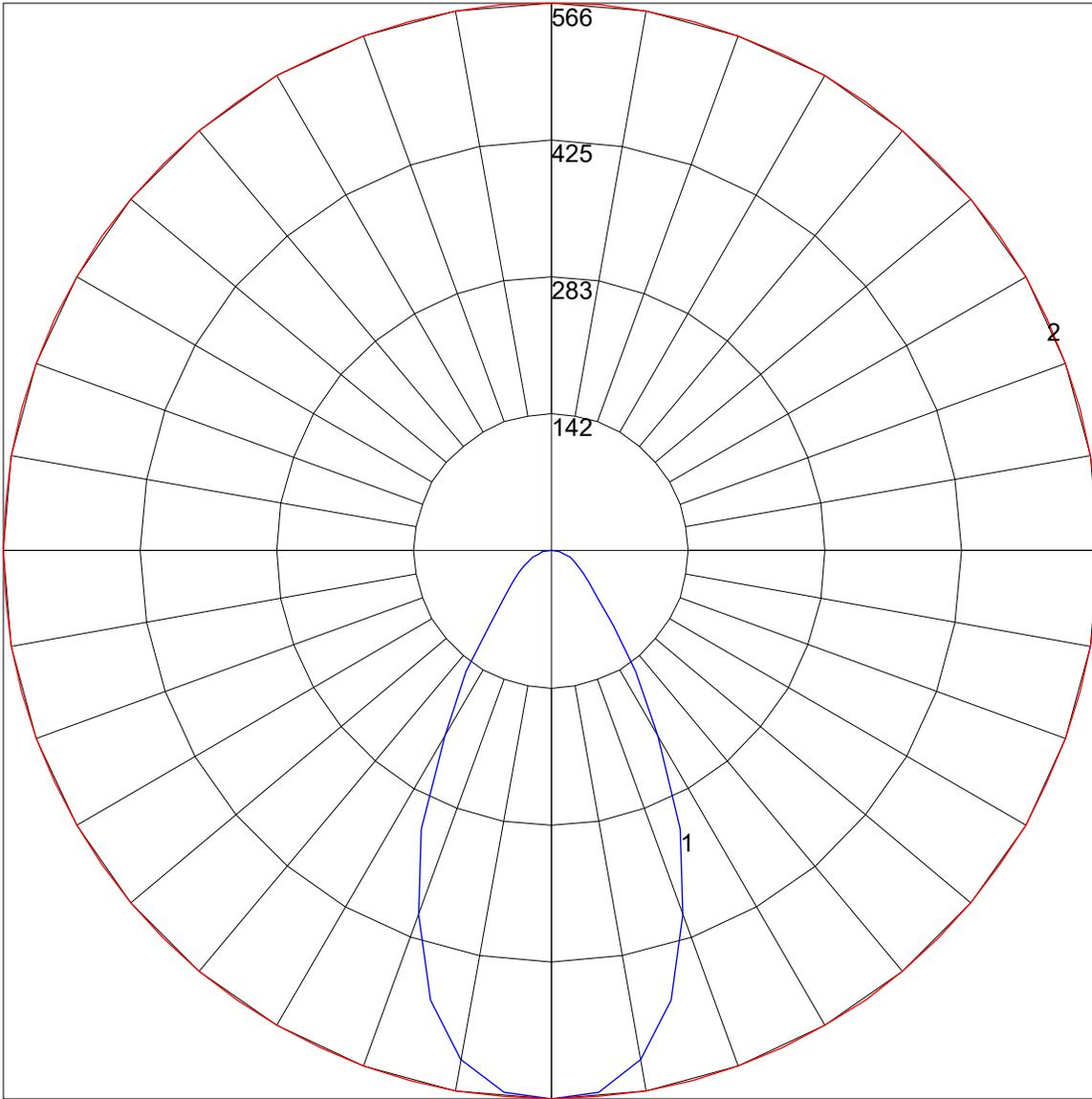
Maximum Candela = 566.4 Located At Horizontal Angle = 0, Vertical Angle = 0
