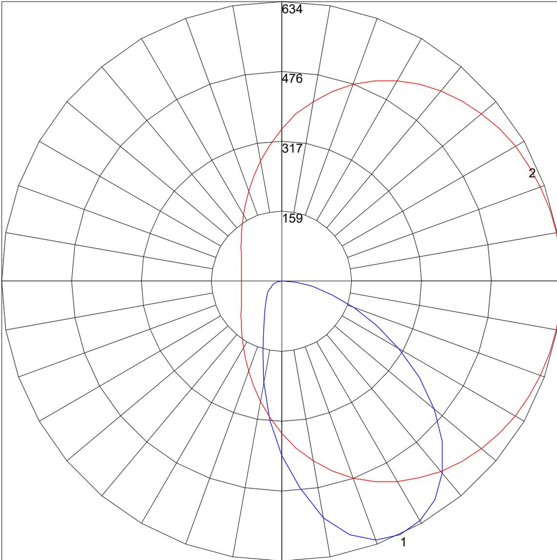
Maximum Candela = 634.15 Located At Horizontal Angle = 0, Vertical Angle = 25
